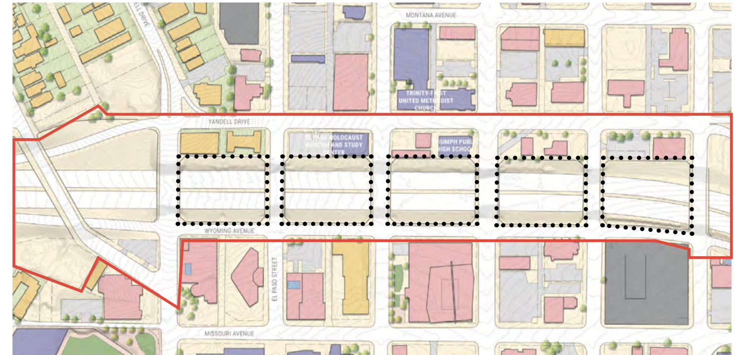
Plan of existing conditions showing the proposed decked areas and the right-of-way for the I-10 study.
